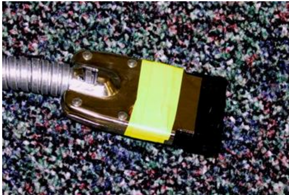
Picture 9-15 Completed Color Coding of Cable Assembly
